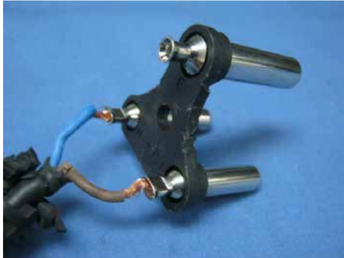
Internal view of the plug without earthing cords for earthing pin
