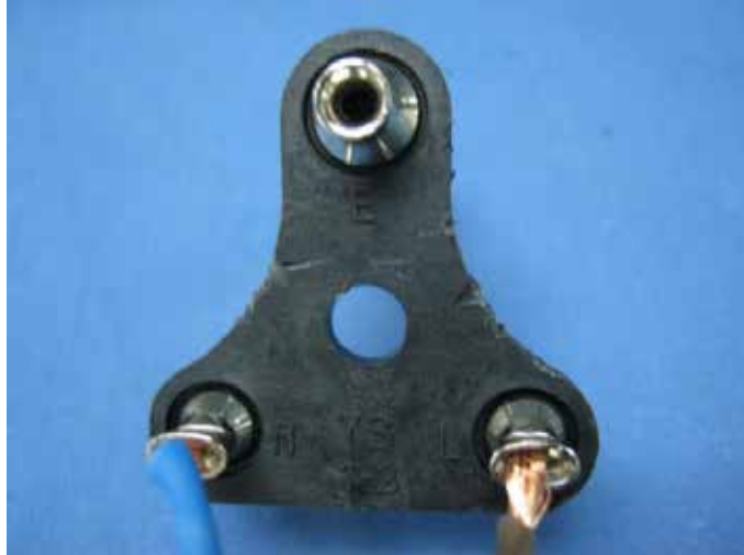
Internal view of the plug without earthing cords for earthing pin
