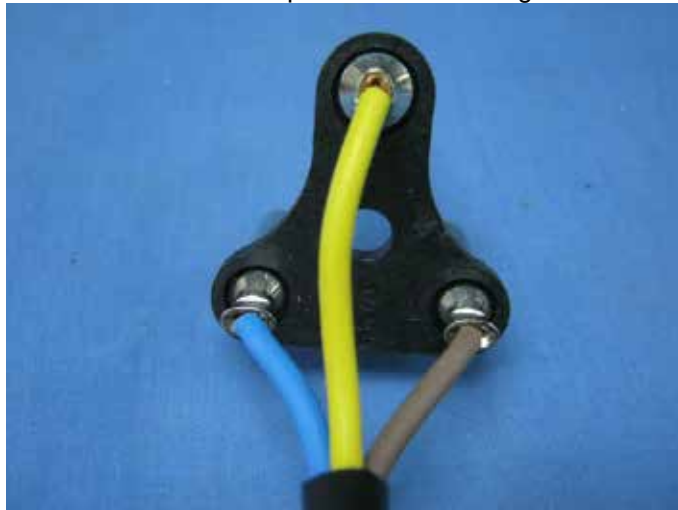
Internal view of the pin without insulating sleeves
